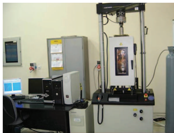
Figure 10. Fatigue test in the climatic cabinet. [Color figure can be viewed in the online issue, which is available at wileyonlinelibrary.com .]
