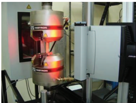
Figure 3. Experiment with the video extensometer. [Color figure can be viewed in the online issue, which is available at wileyonlinelibrary.com .]
